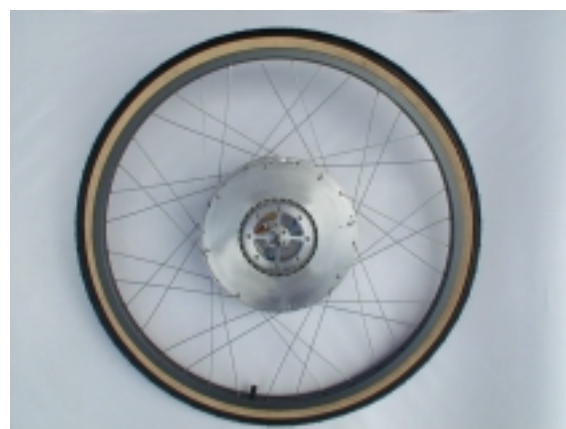
Figure 2: Front wheel with integrated motor
