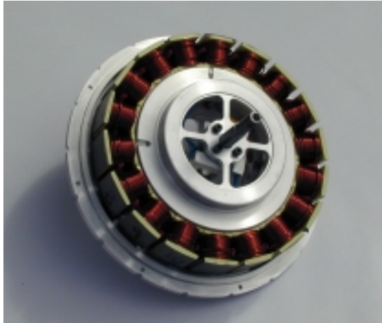
Figure 4: Stator of the new motor
